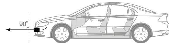
**S8 antenna** must face outward and parallel to the road
